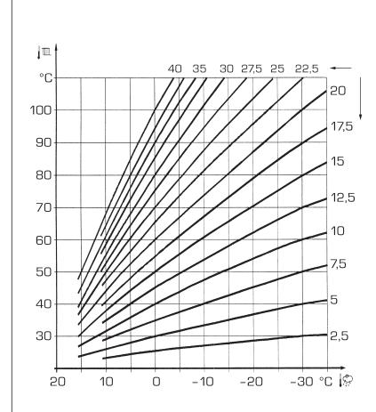
ATTENTION: curves are calculated at an ambient temperature of 20°C. The user can act on the boiler controls to change the environment set for which the bend has been calculated by  $\pm 5$ °C.
