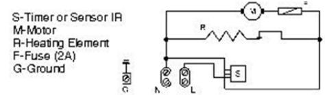
Note: Fuse placed in the PC board.
