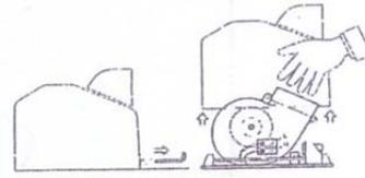
1.c) Set the base on the wall, after drilling it with four holes Ø 8, using the template provided, screwing the screws provided in the hardware bag. See in the template, recommended mounting heights.
